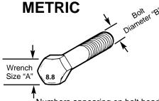
Numbers appearing on bolt heads indicate ASTM class.
